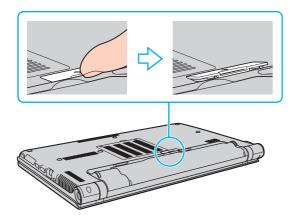
You may find it difficult to remove the port replicator connector cover, as it is tight in place on your computer. Do not exert extra pressure when removing the cover so as not to damage the computer or the port replicator connector cover.
